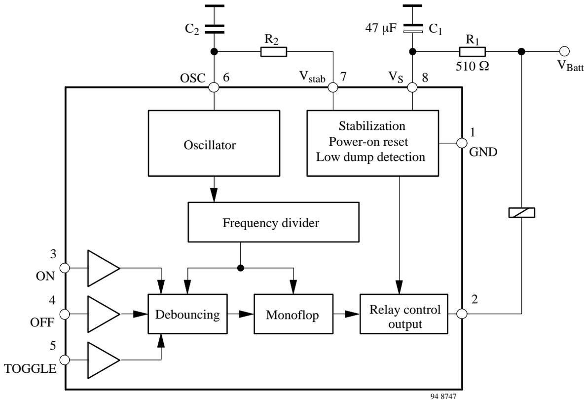
Figure 1 Block diagram with external circuit
